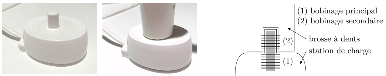
Figure 9 Station de charge
